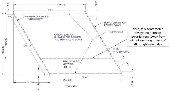
Note: Most of the details in this manual are referencing 30 degree parking angle to the right if on the street facing the curb. This system can be used for left angle parking as well by simply turning over canopy so edge seams are facing up. All dimensional information would simply be mirrored.
