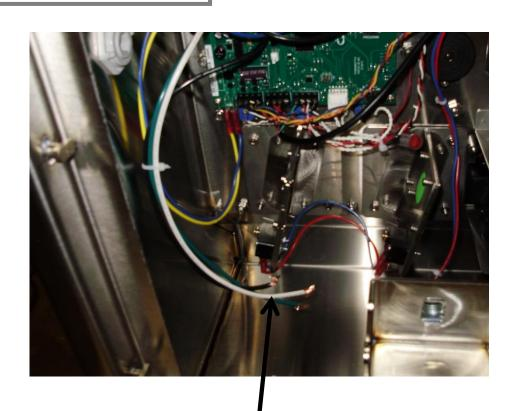
• If unit has water push out knockout in right lower side of unit and plumb water thru and into solenoid inside machine.
