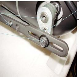
FOR 45 DEG OPERATIOM REMOVE MAIN SCREW AND POSITION BRACKET TO CENTER HOLE. ATTACH HARDWARE AS REMOVED.
